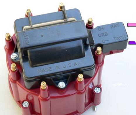
[ENGINE SECTION] #920 TO COIL + (IGN. POWER)
